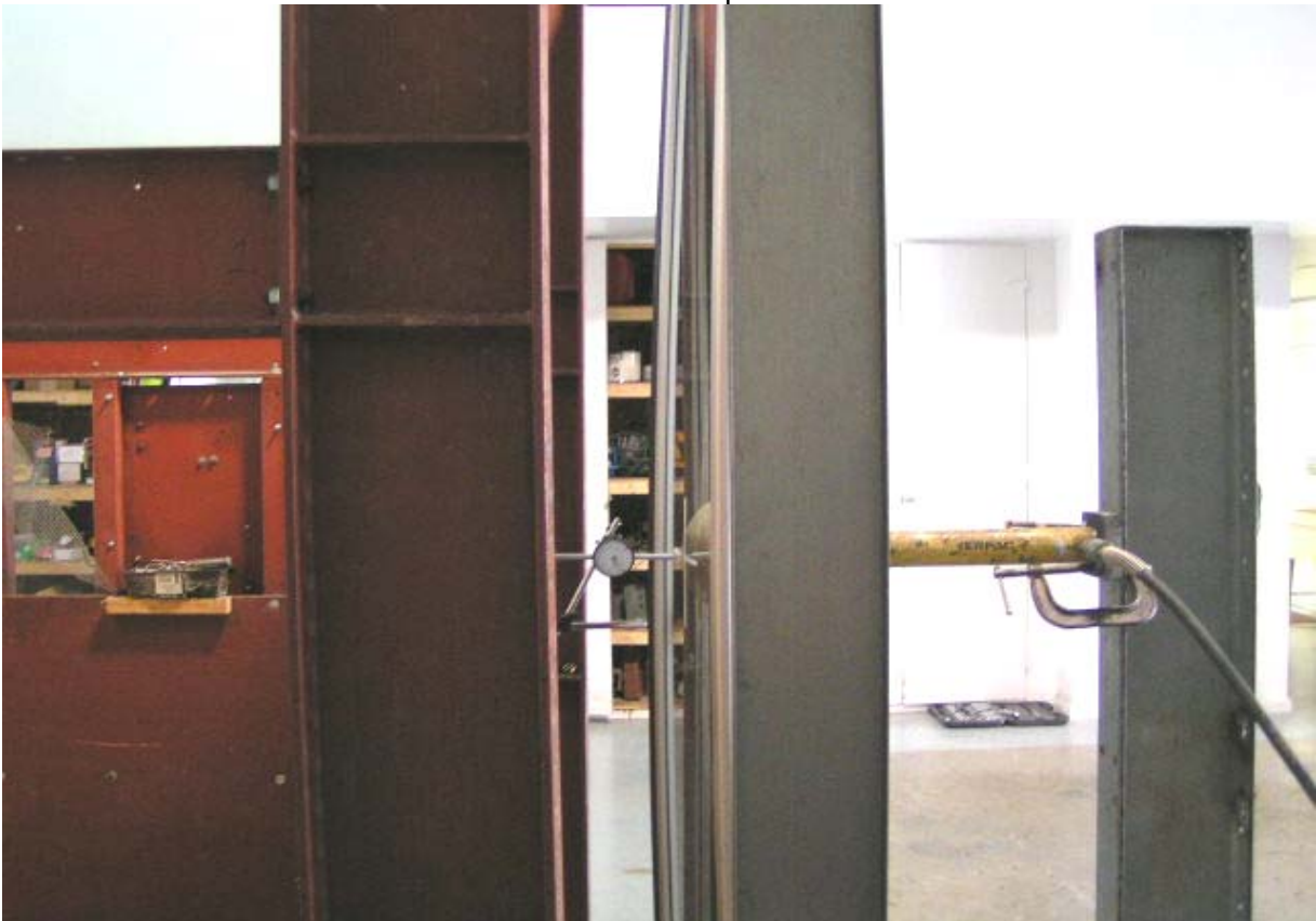
Entry Door #1 When Allowable Deflection Was Met
