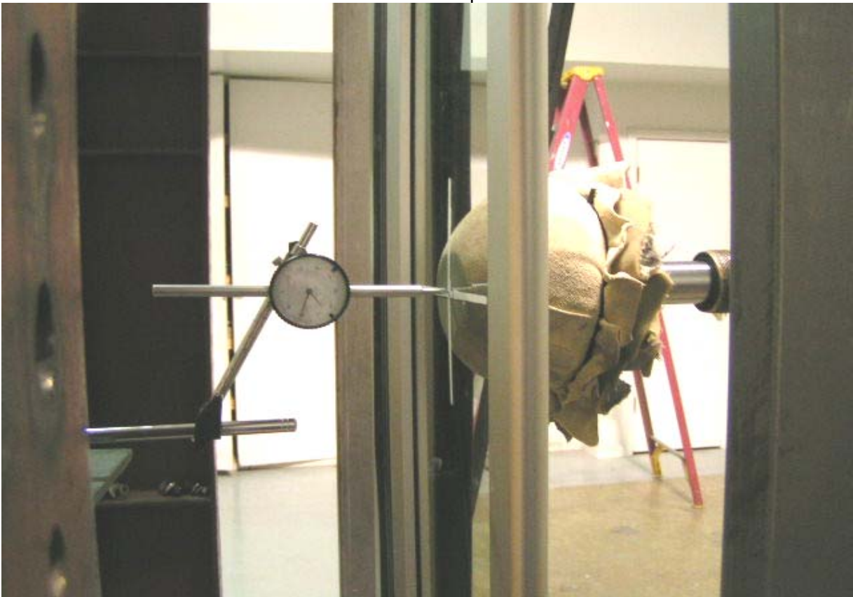
Entry Door #2 When Allowable Deflection Was Met
